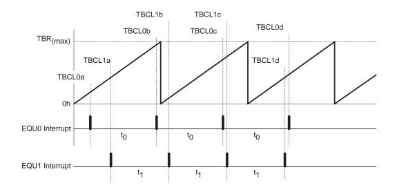
Time intervals can be produced with other modes as well, where TBCL0 is used as the period register. Their handling is more complex since the sum of the old TBCLx data and the new period can be higher than the TBCL0 value. When the sum of the previous TBCLx value plus  $t_{\rm X}$  is greater than the TBCL0 data, the old TBCL0 value must be subtracted to obtain the correct time interval.
